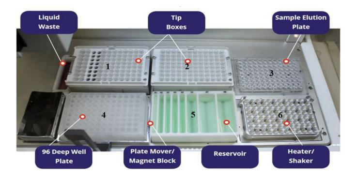
FIGURE 2. Deck layout of VERSA 10
